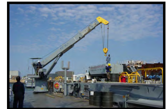
LCU Salvage Deck Crane
