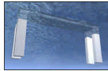
Figure 2. Spar Hull Configuration (underwater view)
